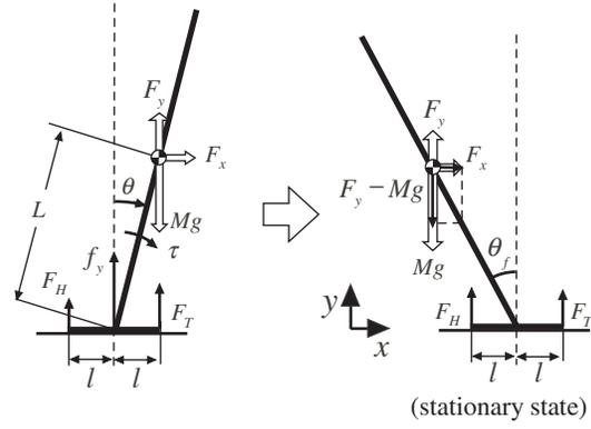
Fig. 2. Link model for static balancing.
