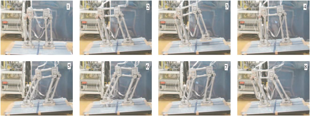
Fig. 5. In-place stepping motion experiment of the slope.
