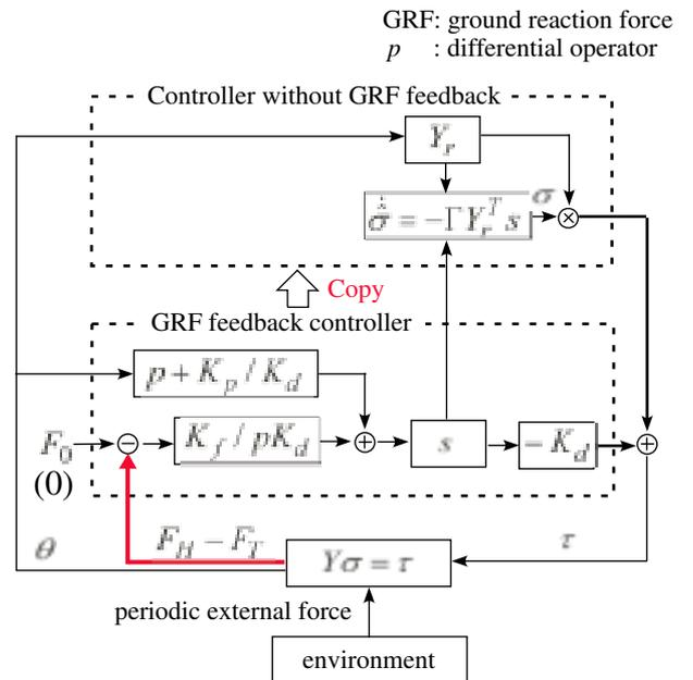
Figure 6: Block diagram of control scheme.
