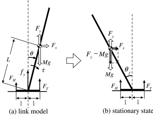
Figure 1: Model and stationary posture by proposed control law.
