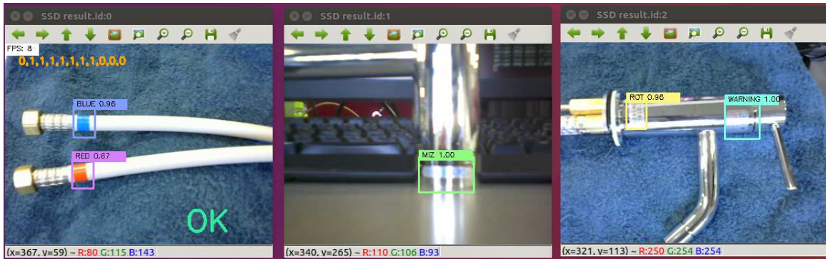
Fig. 5 The inspection Test using three webcams.
