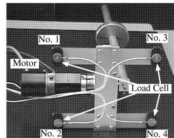
(b) Four loadcells on the sole.
