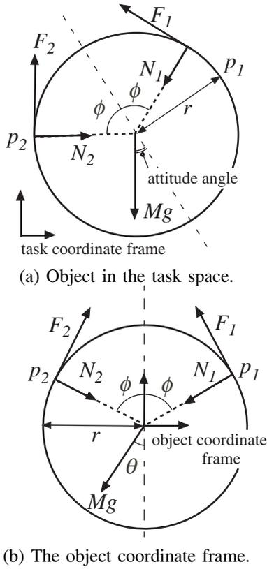
Fig. 1. Grasping of a circular object.
