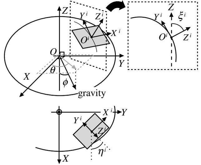
Fig. 3. Contact-point coordinate frame.
