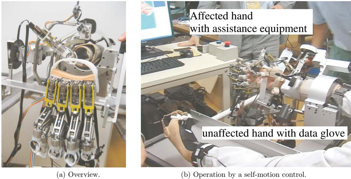
Fig. 1. A hand rehabilitation equipment with 18 DoFs.
