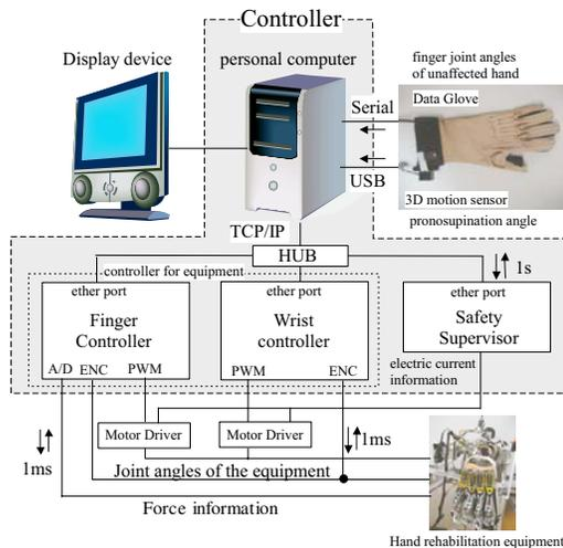
Fig. 2. Controller structure.
