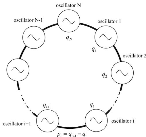
Fig. 2. A circularly coupled oscillator system.
