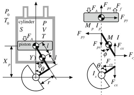
**Fig. 5.** Mechanical model of engine.
