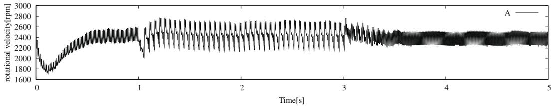
(a) Rotation velocity of the engine shaft.
