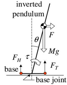
Fig.2. Simple biped model
