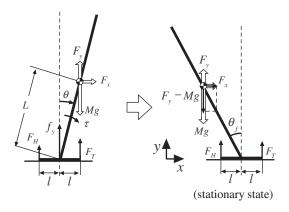
Fig. 2. Link model for static balancing.
