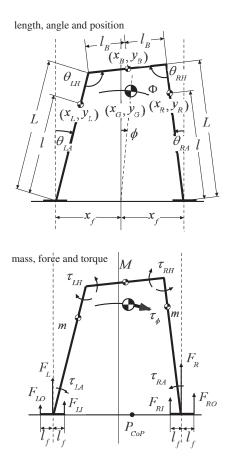
Fig. 3. Link model for motion control in double support phase .
