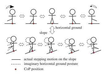
Fig. 1. Lateral stepping motion on different gradient condition.
