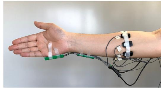
Fig. 2 Electrodes attached around the forearm with the same intervals.
