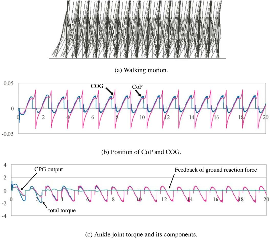
Figure 5: Simulation of walking motion without external force.
