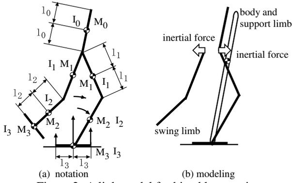
Figure 2: A link model for biped locomotion
