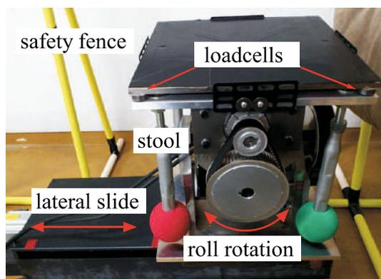
**Fig. 2** Stool with lateral slide and rolling movements
