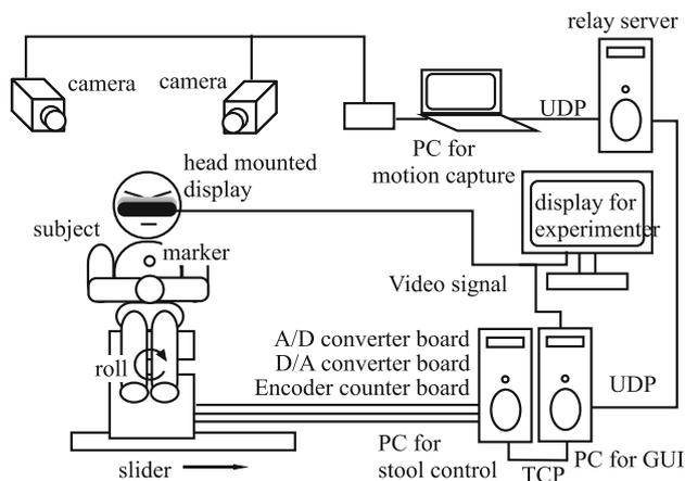
**Fig. 8** Setup for human experiments
