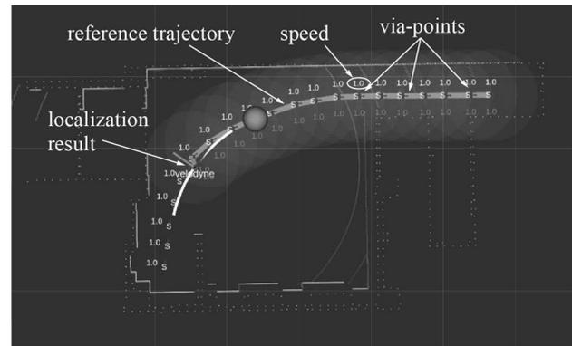
**Fig. 8** Reference trajectory (a bold dark line) and localization result on the created PCD map. About 20 plotted via points designate the reference trajectory by interpolating them. The numbers near the via points denote the speed there
