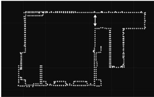
**Fig. 4** PCD map downsampled by the 2D VGF
