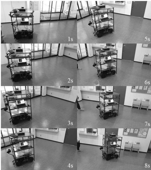
Fig. 9 Snapshots of the AMR movement
