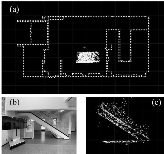
**Fig. 5** PCD map where an obstacle PCD is overlaid
