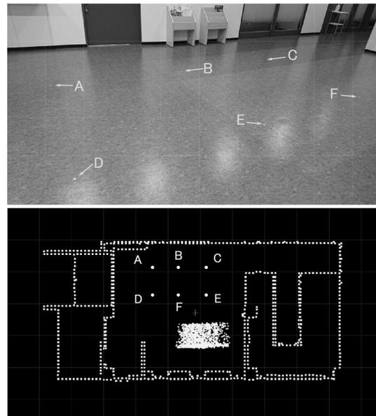
Fig. 10 Six test points, A–F, in the experiment. Top: six points’ position on the photo and bottom: their position on the PCD map
